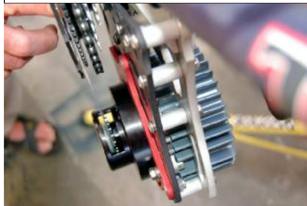
(11) Checking Sprocket Alignment
