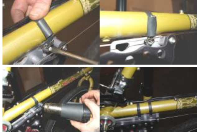
(7) Tighten Adjustable Clamps, Feeding Excess Into Shrink Wrap
