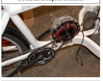
(8) Installing the Motor Chain
