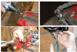
(8A) Adjusting Length and Pulling Chain Ends Together
