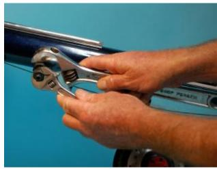
(5C) Wrench Type Rivet Nut Tool
