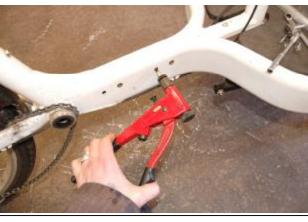
(5D) Lever Type Rivet Nut Tool
