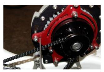
(8D) Using Set Screws to Align Motor Chain
