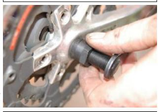
(2) Removing Crank with Crank Puller
